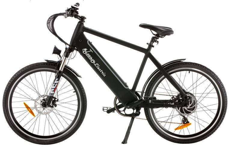
Motor: 500W 48V high-speed geared-hub motor in rear wheel
