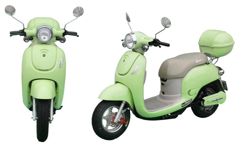
Motor: MOTORINO CCT 500W Nominal power 48V brushless, Max torque: 66 Nm Motor Controller: 18 MOSFETs MOTORINO CCT Sine-Wave with regenerative braking Battery: Removable 48V 20A-h sealed lead-acid / 48V 26A-h Lithium Ion (LiFePO4)
