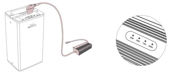
5 When the battery is fully charged, the charge indicators are all green.
