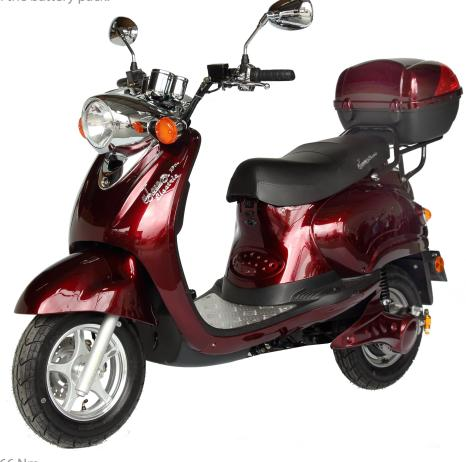
Motor: MOTORINO CCT 500W 60V brushless, Max torque: 66 Nm
