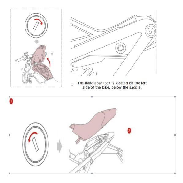
1. Insert the key and rotate it rightwards, and the storage box will be opened when you hear a [Click] sound.
