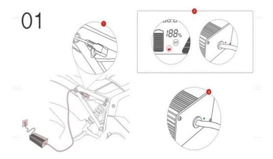
How to charge the battery on the bike
