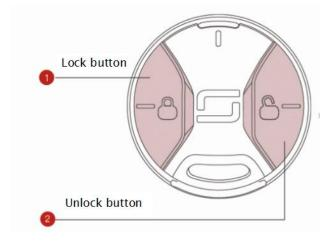
1. Lock button. When the bike is in the [Static State], press the lock button, and the start button flashes. The bike enters the [Locked State].
