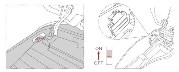
TIPS: In order to protect your safety, please turn off the air switch when cleaning, storing the bike for a long time, or removing the battery pack.
