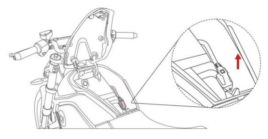
3. Insert the key into the anti-theft battery lock and rotate it rightwards to remove the battery from the bike.
