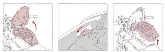
1. Open the storage case, close the air switch and take out the storage box.
