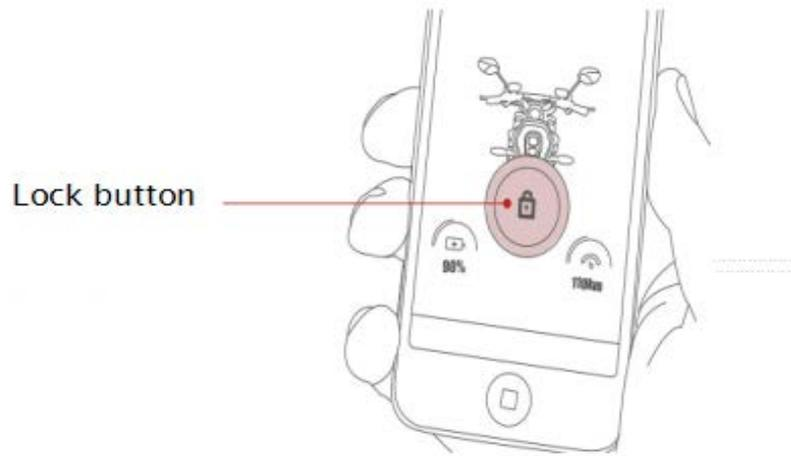
**Lock button:** when the bike is in a [Static State], press the lock button, and the start button will flash. The bike enters the [Lock State]
