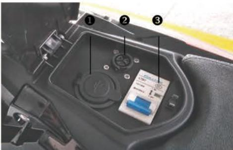
The main circuit breaker ❸ is the protection switch of ES1 PRO main power supply. When the current caused by abnormal or short circuit of the motorcycle exceeds the safety setting value, the air switch will be automatically disconnected to ensure safety.
