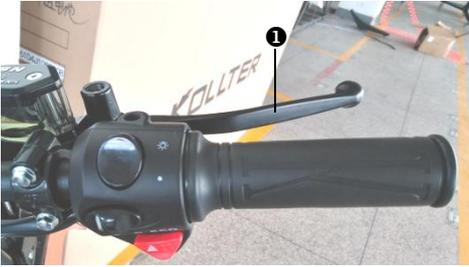
The front brake handle ❶ is fitted on the right side of the handlebar.
