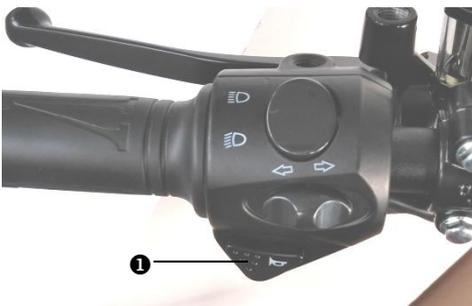
When the key is in the ON position, the horn sounds when the button ❶ is pressed. the horn can be used to warn pedestrians or other motorists of your presence.
