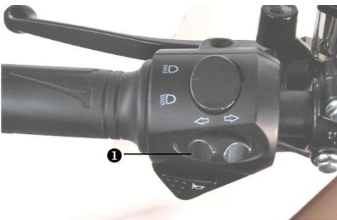
The steering lamp switch ❶ is on the left handle switch.
