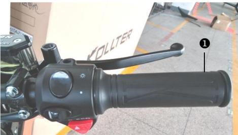
The throttle grip ❶ is fitted on the right side of the handlebar.
