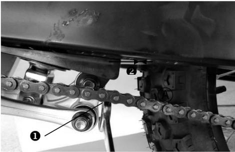
Push the chain at the lower end of the chain support ❶ upward to check the tension of the chain between the chain and the chain support.
