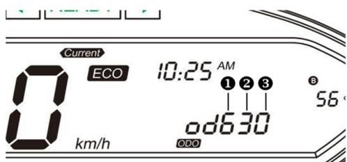
After setting the minute of the time, press the adjustment button again for a long time. The hundreds place ❶ of the front tire diameter will start flashing, and the short press will cycle between 0 and 9.
