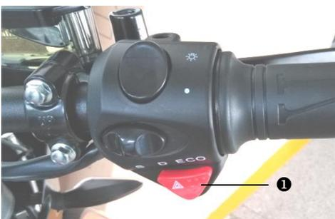
When the button ❶ is pressed, the turning lights flash to warn other drivers of situations, which include stop or park under emergency conditions.
