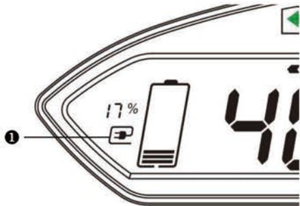
During cycling, when you brake the vehicle, the controller recovers the braking energy. At the same time the charging symbol ① will light up.
