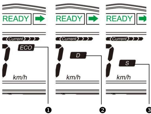
The riding mode is a shift switch located on the right-hand handle switch
