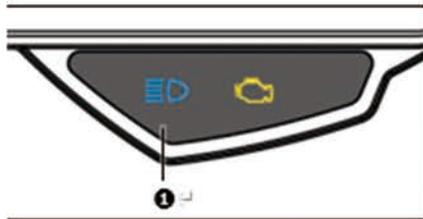
When the headlight high beam is on, this indicator <sup>①</sup> illuminates blue, and remains on until the high beam is turned off.
