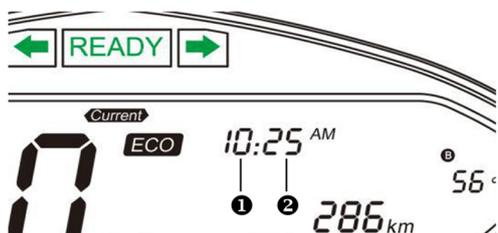
Press and hold the adjustment button at the back of the instrument panel, then switch on to enter the setting interface.
