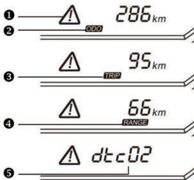
When the error code indicator <sup>①</sup> turns on, it indicates a fault in the motorcycle. The error code is displayed in the odometer.
