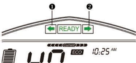
An arrow on the upper speedometer flashes green in the same direction as selected by the steering lamp switch. This remains flashing until the steering lamp request has been canceled.
