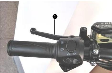
The rear brake lever ❶ is fitted on the left side of the handlebar.
