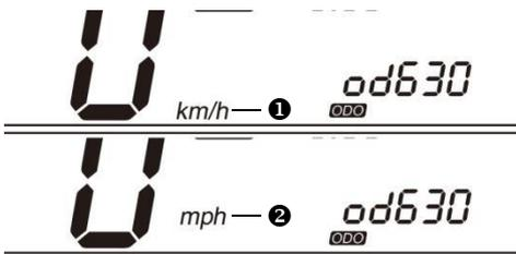
After setting the front tire diameter parameter, press and hold the adjustment button again to enter the MM/INCH setting.
