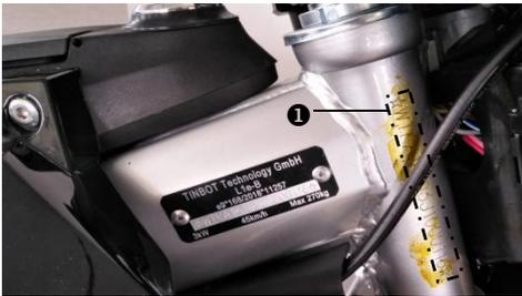
The chassis number ❶ is stamped on the right side of the steering head.
