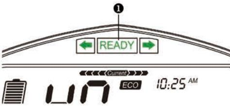
“READY”<sup>①</sup> indicates that the HV system is connected and the motorcycle is ready to ride, while the speed is 0 km/h.
