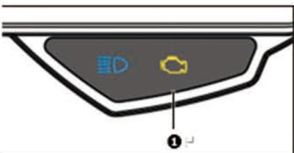
OBD trouble light When the OBD trouble light is on, it indicates that the vehicle has a running fault. Please go to the dealer for inspection.
